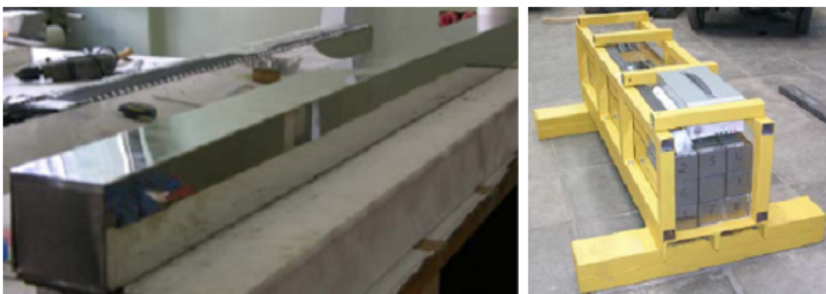
Fig. 43: Fully assembled module (left) and assembled supermodule (right) before the transportation to CERN.
