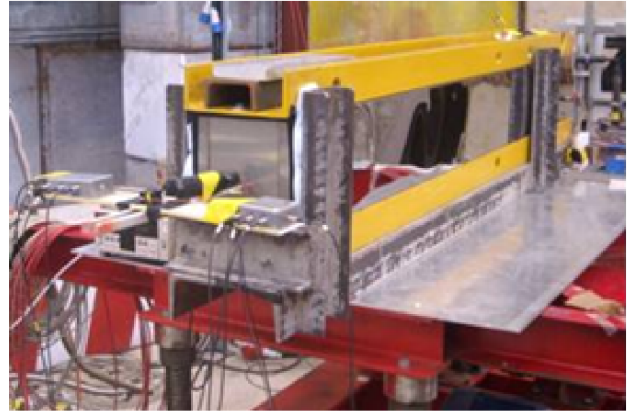
Fig. 53: Test setup with a large PSD module at the CERN T10 PS beam line.
