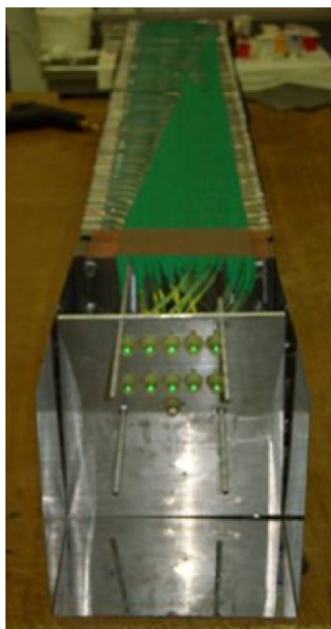
Fig. 22: Photo of an assembled large module.
