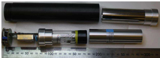
Figure 1: The components of the LaBr 3 detector.
