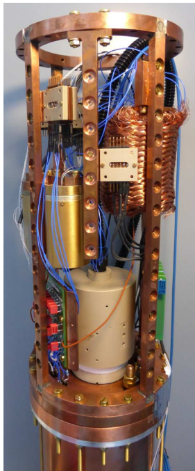
Figure 1: Photography of the ARTEMIS trap chamber with the electronics, for example ion motion detection circuits, laser inlet and filterboards.
