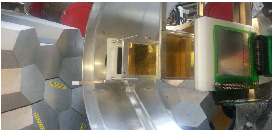
Figure 6.46.: Targets for experiment S426 mounted in the PreSPEC-AGATA setup. The beam ions enter from the right. Their transverse position is measured in the target DSSSD (green PCB frame) before they impinge on the first gold target at the nominal target position in the focus of the AGATA detectors. This target has a thickness of 2 \text{ g/cm}^2 . The second target with a thickness of 1 \text{ g/cm}^2 is mounted 10 cm further downstream. The quadratic targets have an edge length of 10 cm. See text for details.
