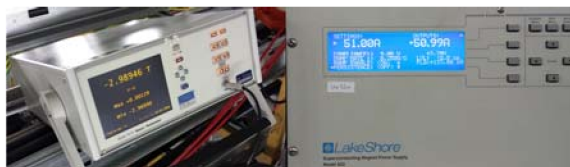
Figure 1: Magnetic field of 3 T and corresponding electric current (51 A) in the superconducting magnet during the test. The cold magnet kept its field in persistence mode i.e. after the current power supply was switched off.
