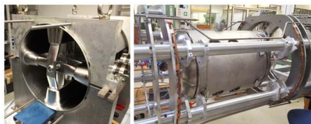
Figure 2: Superconducting 217 MHz CH cavity during manufacturing (left) and finally mounted into the support frame of the horizontal cryomodule (right) [2].
