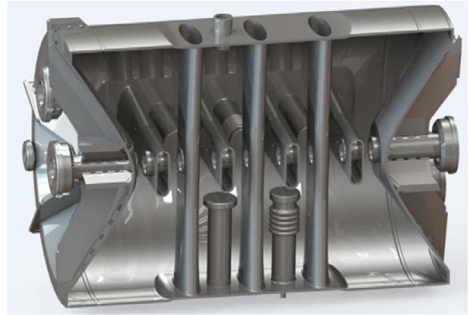
Figure 1: Final design of the sc 217 MHz CH-cavity.
