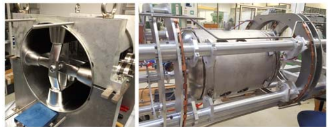
Figure 2: Superconducting 217 MHz CH cavity during manufacturing (left) and finally mounted into the support frame of the horizontal cryomodule (right) [2].
