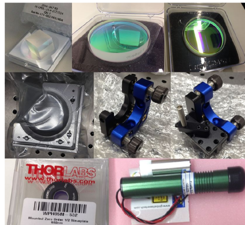
Figure 1: Collage showing a selection of the components purchased in 2016. Top row, polarizing beam splitter cube and doubly-coated mirrors. Middle row, mirror mounts (vacuum, 2", prism). Bottom row, \lambda/4 -plate, green laser.
