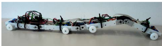
Figure 1: Fully functional prototype model of the SIS100 inspection robot.
