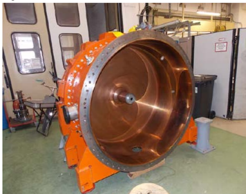
Figure 1: A UNILAC single resonator cavity is under modification for smoothing the micro spill structure.
