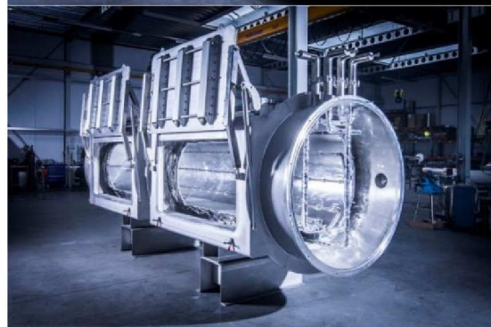
Figure 6: Universal cryostat for FAIR components testing
