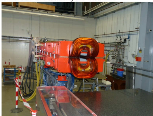
Figure 2: dip13_0 during magnetic measurement at GSI
