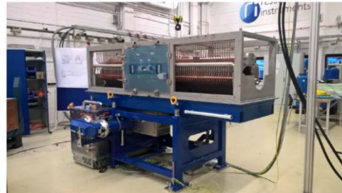
Figure 3: First of Series (FOS) SIS100 acceleration cavity at factory acceptance test at Research Instruments (RI).
