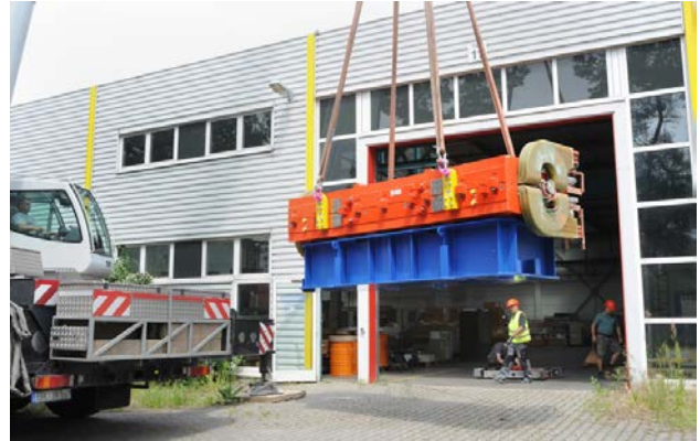
Figure 9: Unloading of one HESR dipole magnet (weight: 35t) at the site of an external storehouse
