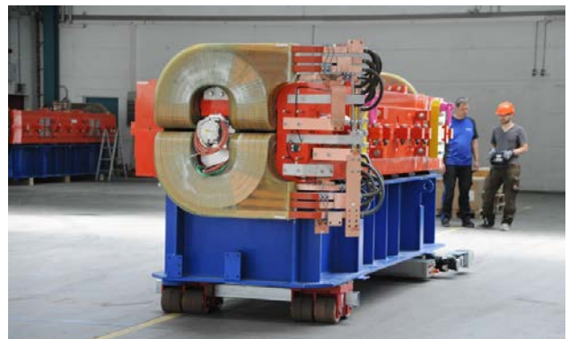
Figure 10: Remote positioning of an HESR dipole magnet for intermediate storage.
