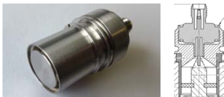
Figure 2: Button pickup from NTG. Diameter 12 mm, gap width between button and housing 1.5 mm.
