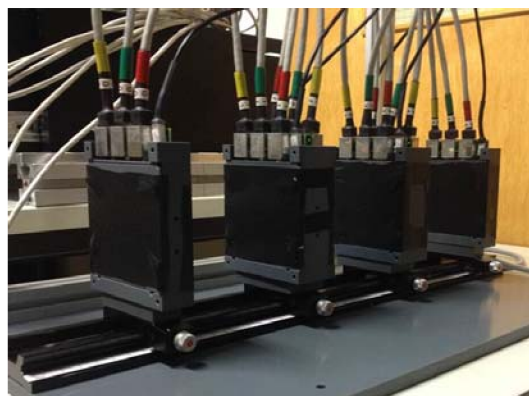
Figure 2: 6 MIMOSA28 sensors placed the optical bench.
