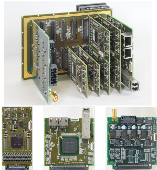
Figure 1: A 3x2 MAPMT readout module (top), with one out of 6 MAPMTs on front side, and few 32ch DiRICH FPGA-TDC frontend modules (lower left), a DiRICH-Power supply module (lower right), and a DiRICH-Combiner module (lower center).
