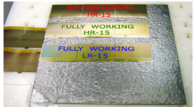
Figure 1: Configuration of sensors assembled on the front side of the PRESTO module. First side assembled with sensors and flex cables.
