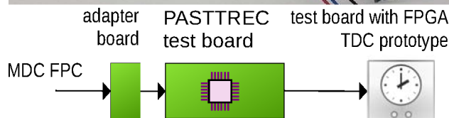
Figure 1: PASTTREC read-out line, here equipped with a stand-alone FPGA-based prototype TDC.
