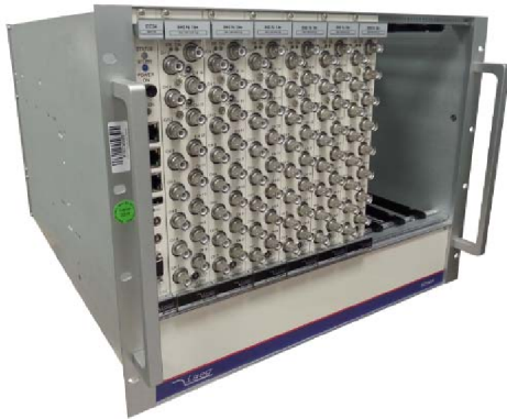
Figure 1: The ISEG crate with 6 modules à 16 channels and a CC24 master.
