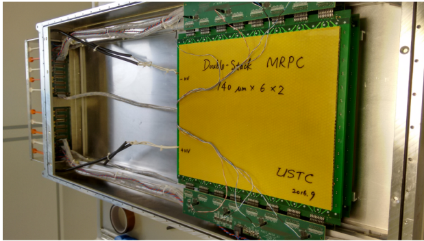
Figure 3: View inside the open STAR CBM TOF module.
