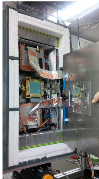
Figure 1: Thermal enclosure with cooling lines at the perimeter of the core part and two ALIBAVA daughter boards.
