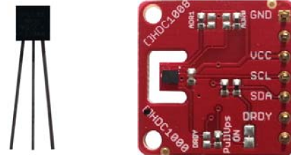
Figure 3: left: One DS18B20 1-wire sensor from Maxim Integrated. right: A HDC1000 sensor on a breakout board.
