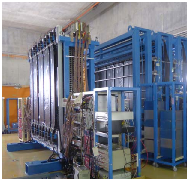
Figure 4: The downstream area of the SAMURAI setup. The NeuLAND demonstrator, equipped with a VETO detector from RIKEN, is located in front of NEBULA. Neutrons impinging on NeuLAND come from the left.
