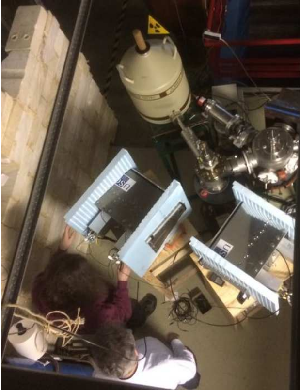
Figure 1: Top view of the experimental setup during the experiment at the Tandem accelerator of the CTN/IST laboratory. The reaction target, at the end of the beam line, is surrounded by the two CALIFA petals used in the experiment, as well as the HPGe detector.
