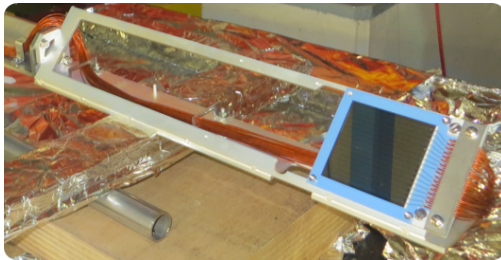
Figure 1: A photo of the UHV compatible DSSSD used in the experiment.
