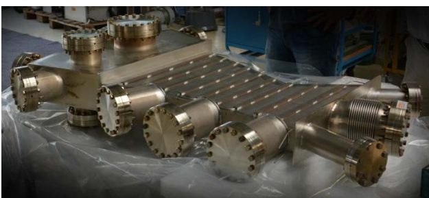
Figure 2: The new dipole chamber at first inspection in the UHV lab of GSI before the vacuum tests.
