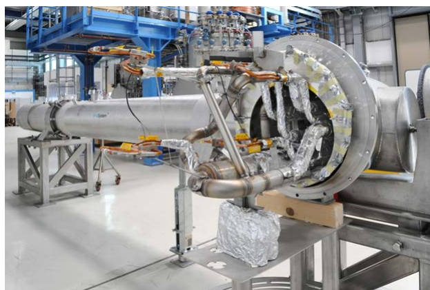
Figure 6: First-of-Series cryogenic bypass line of the local cryogenic system of SIS100 installed at the GSI Series Test Facility
