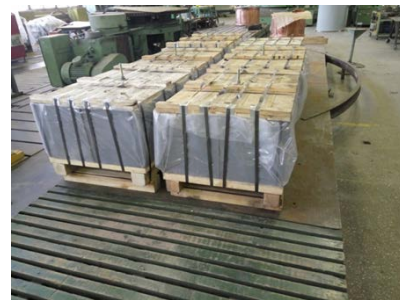
Figure 11: Lamination for dipole magnet dip15_0 at BINP
