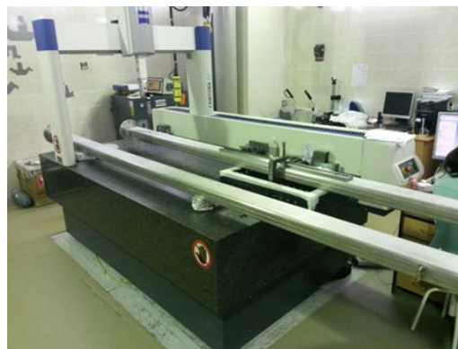
Figure 14: Geometrical inspection of pre-series chambers during FAT at BINP in May 2017
