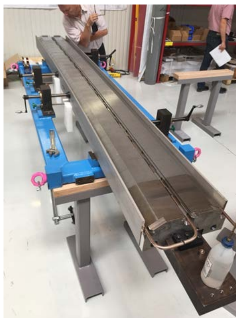
Figure 4: Yoke manufacturing for the series dipole magnets
