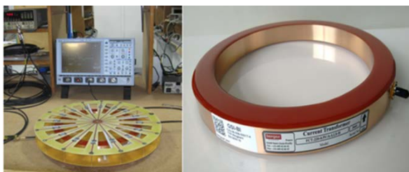
Figure 12: Current transformer of FCT
