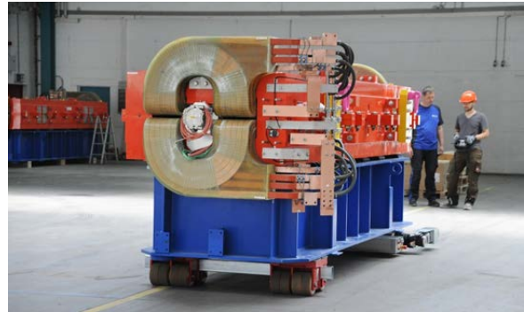
Figure 22: Remote positioning of an HESR dipole magnet
