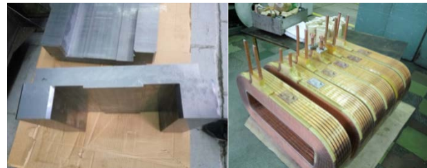
Figure 10: Yoke halves (left) and coils (right) of the steering magnet s100
