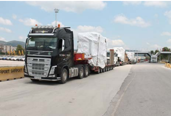
Figure 17: Transformers ready for transport
