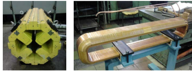
Figure 9: Yoke (left) and coil of the quadrupole magnet quad2 (right)
