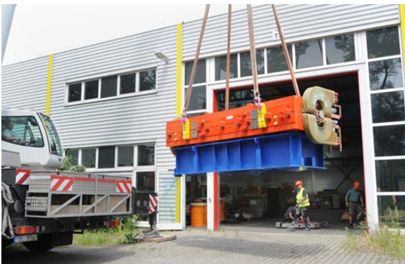
Figure 21: Unloading of one of the HESR dipole magnets
