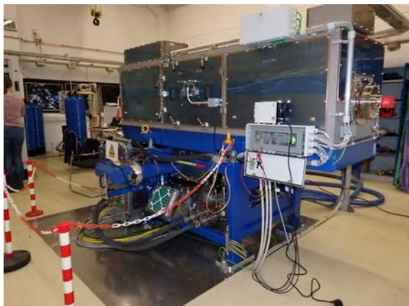
Figure 5: First-of-Series radiofrequency accelerator cavity at external company site.
