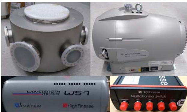
Figure 1: Collage showing a selection of the components purchased in 2017. Upper row: vacuum chamber ‘mirror box’, rotary fore-pump. Lower row: high-precision wavelength meter, multichannel switch (for 4 laser systems).
