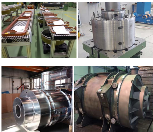
Figure 1: FoS short multiplet manufacturing: quadrupole and sextupole coils (upper left panel), sextupole yoke assembly (upper right panel), thermal shield (lower left panel), and vacuum vessel (lower right panel).
