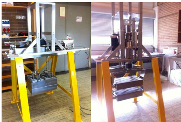
Figure 1: X-slit first of series of Super-FRS X- (left panel) and Y-slits (right panel).
