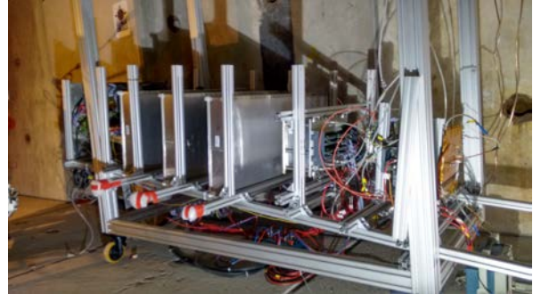
Figure 1: Photography of the CERN November 2016 setup. The beam enters the setup from the right side. The counters are arranged below the beam with an angle of 7°.
