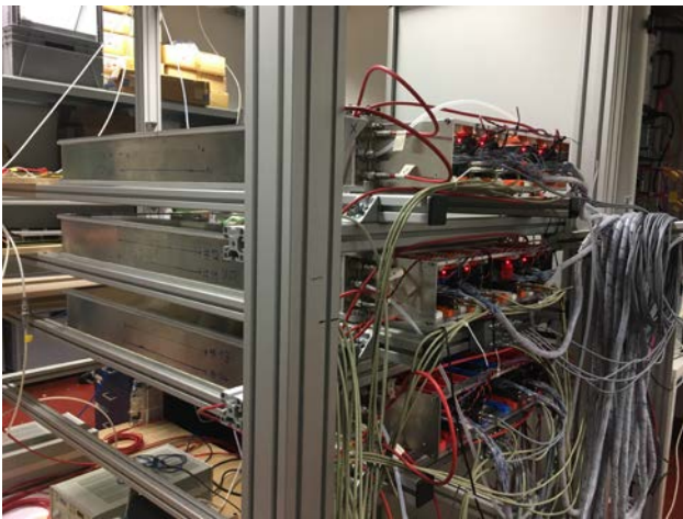
Figure 2: Photography of the Heidelberg cosmic setup. Three modules containing 2 counters each are placed on top of each other so that in total 6 counters can be tested simultaneously.
