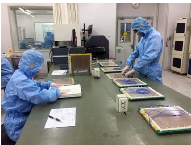
Figure 4: Mass production of MRPC3a counter in the clean room.
