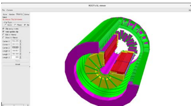
Figure 5: eTOF geometry included in the STAR simulation framework.
