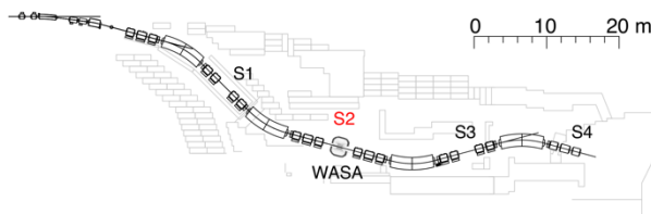
Figure 1: Layout of the FRS. The WASA CD will be mounted at the mid-focal plane S2.
