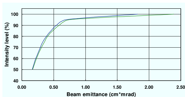
Figure 2: Beam intensity inside a given total beam emittance behind the RFQ channel, calculated from the results of the codes BEAMDULAC (green) and DYNAMION (blue).
