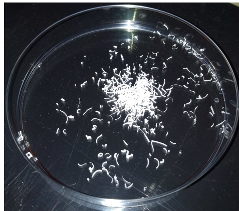
Figure 5.3.: Photograph of the polystyrene granulate supplied by the manufacturer.
