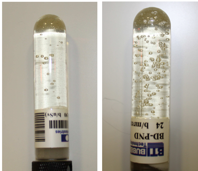
Figure 4.2.: Photograph of a bubble detector irradiated with a low neutron dose (left) and one irradiated with a high neutron dose (right).
