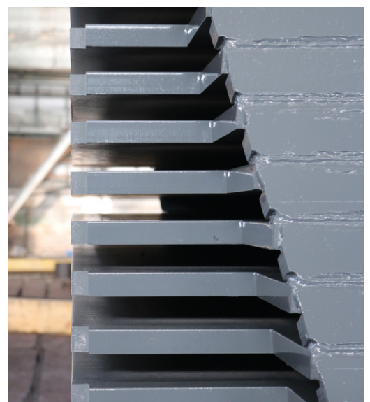
Figure 29. Left: First octant of the iron yoke for the PANDA Solenoid Magnet. Right: Rear part of the iron yoke for the PANDA Solenoid Magnet.
