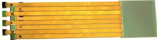
Figure 8: First copper module completely assembled with STS-XYters on N- and P-side.
