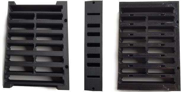
Figure 5: 3d-printed ABS plastic mask for direct backplane and indirect readout electronics air cooling (left to right; top, side and bottom view)
