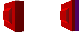
Figure 1: First absorber of Muon Chamber. Left panel: 60 cm high density carbon ( \rho = 2.26 \text{ gm/cm}^3 ). Right panel: 30 cm low density carbon ( \rho = 1.7 \text{ gm/cm}^3 ) + 30 cm concrete ( \rho = 2.3 \text{ gm/cm}^3 ).
