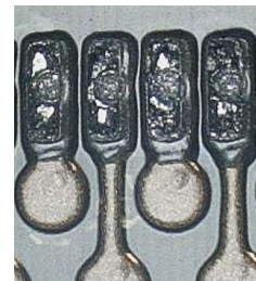
Figure 6: Perfectly centered imprints of the Au stud bumps from the sensor side in the solder depot of the cable.
