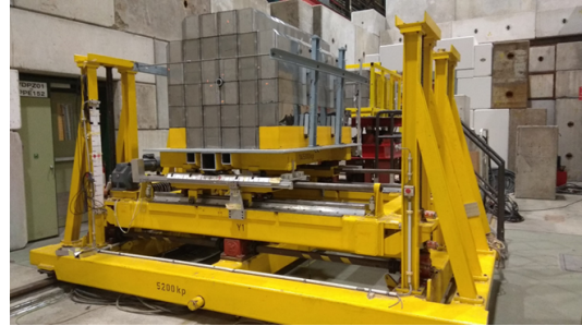
Figure 2: The upgraded NA61/SHINE mPSD which used 13 CBM PSD modules. First experiments at BM@N and NA61/SHINE are expected at the end of 2021.
