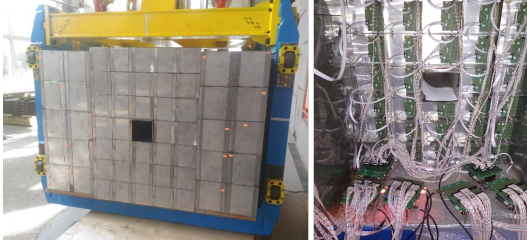
Figure 1: Left - front view of the BM@N FHCAL. Right – the backside of the FHCAL with installed FEE and readout electronics.
