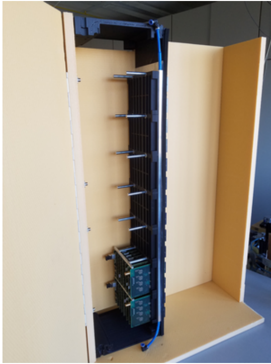
Figure 4: Cooling system prototype with seven 3 \times 2 MAPMT readout modules
