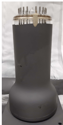
Figure 8. Conductive coating on the PMT together with the interconnecting line.
