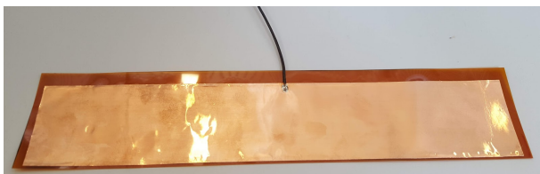
Figure 6. Electrostatic shielding in the expanded form.
