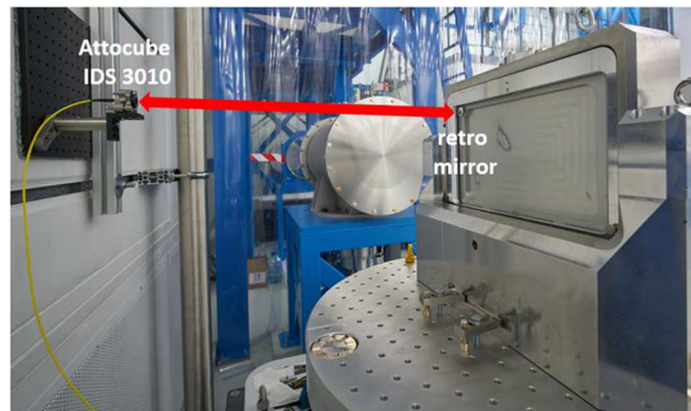
Figure 12. Wall-mounted Attocube IDS 3010 sensor with mirror mount bolted onto its breadboard installed on the chamber base plate and granite block L3-E3-F040.
