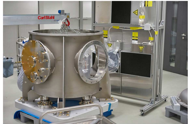
Figure 21. Assembly of HAPLS BT vacuum vessels and optomechanics in cleanroom class ISO 5.
