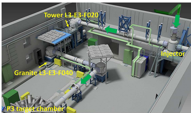
Figure 4. 3D CAD visualization of the HAPLS BT from the injector chamber to the P3 chamber. This figure shows the actual installation in E3.
