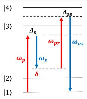
**Figure 1.** Schematic of CARS, where an anti-Stokes signal is generated by the four-wave-mixing process. Maximizing the coherence between states  $|1\rangle$  and  $|2\rangle$ ,  $\rho_{21}$ , is the key to amplifying the signal response from the system. Here,  $\Delta_s$  and  $\Delta_{as}$  are the one-photon detunings, and  $\delta$  is the two-photon detuning.
