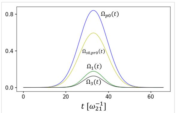
Figure 2. The evolution of different Rabi frequencies in the C-CARS scheme. The Stokes and the probe peak Rabi frequencies  $\Omega_{s_0}$  and  $\Omega_{pr_0}$  have the same amplitude, which is less than the pump Rabi frequency  $\Omega_{p_0}$  by a factor of  $\sqrt{2}$ .  $\Omega_1(t)$  and  $\Omega_2(t)$  are canceled out in the Hamiltonian due to the complete overlap making  $\Omega_3(t)$  the only relevant quantity in the control scheme.
