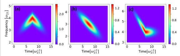
**Figure 3.** Wigner plots of the incident pulses; pump (a), Stokes (b) and probe (c). Note that the Stokes and probe have the same amplitudes, which is different from that of pump. The parameters used in this figure are  $\omega_p = 4.0[\omega_{21}]$ ,  $\omega_s = 3.0[\omega_{21}]$ ,  $\omega_{pr} = 4.0[\omega_{21}]$ ,  $\tau = 3.0[\omega_{21}]$ ,  $\alpha_s = -0.2[\omega_{21}^2]$ , and  $t_c = 7.5[\omega_{21}^{-1}]$ .
