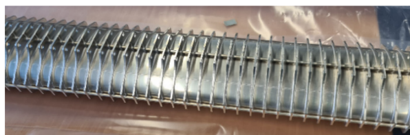
Figure 2: Thin wall, rib reinforced, LHe cooled quadrupole chamber.
