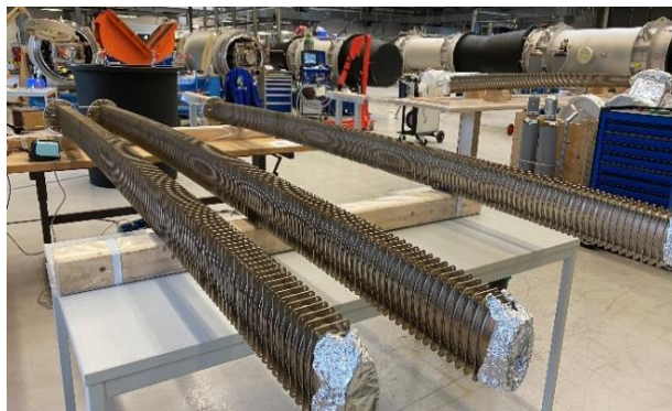
Figure 2: Integration of thin-wall, ripped and LHe-cooled dipole chambers into the s.c. dipole modules (behind).
