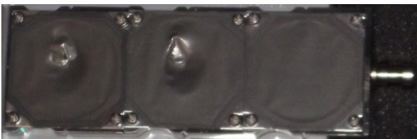
Fig. 3. Carbon foils with 570 µg/cm 2 thickness in the beam diagnostic chamber. The two foils on the left have been irradiated with U 28+ .
