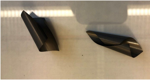
Fig. 1. Carbon foils 570 µg/cm 2 thickness released from glass plate, prepared by standard procedure.
