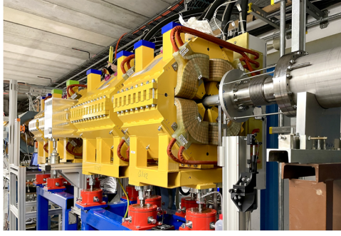
FIG. 6. PRIOR-II setup fielded at the HHT experimental area at GSI. Upstream view from behind the last (short) quadrupole of the imaging quadruplet toward the Fourier plane and the object plane. The last (dark blue) quadrupole of the matching section in front of PRIOR-II (see Fig. 5) can be seen on the left-hand side of the picture.
