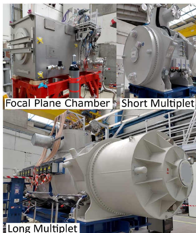
Figure 2: Top-left: Focal plane chamber with an insert and media-board, top-right: superconducting short multiplet, bottom: long multiplet.
