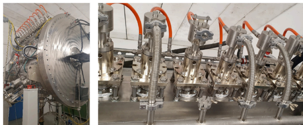
Figure 2: First-of-Series cavity section used for prototyping.
