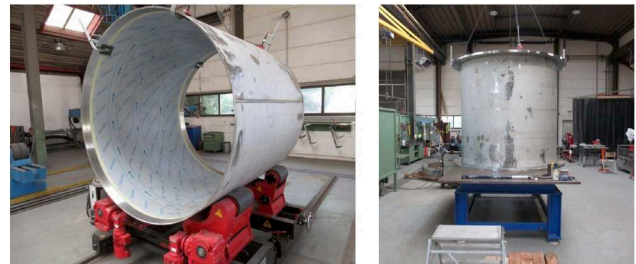
Figure 6: Rolling and welding of a cavity section.
