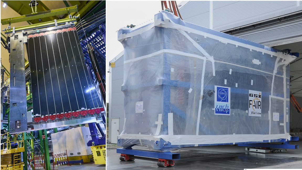
Figure 1. (Left) Single C-frame with 9 straw modules attached on each side, at LHCb/CERN. (Right) Whole OT gaseous tracker in its transport frame, (13.5 \times 5.2 \times 7) \text{ m}^3 , 24 t, arriving at GSI.
