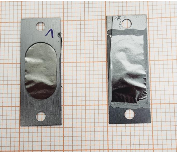
Fig. 3. Self-supported targets of ^{72}\text{Ge} -targets on HORUS-frames with a thickness of \sim 350\text{ }\mu\text{g}/\text{cm}^2 .
