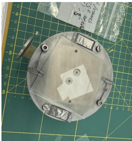
Fig. 1. Sample holder with the mounted glass substrate, already coated with betaine-sucrose in the middle and two target frames with titanium backing attached sideways.
