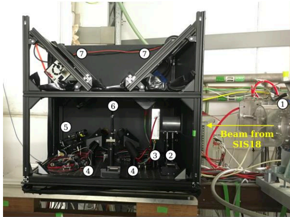
Fig. 2. Photo of the experimental setup for the in-situ characterization of scintillating targets exposed to high energy heavy ion beams [3].
