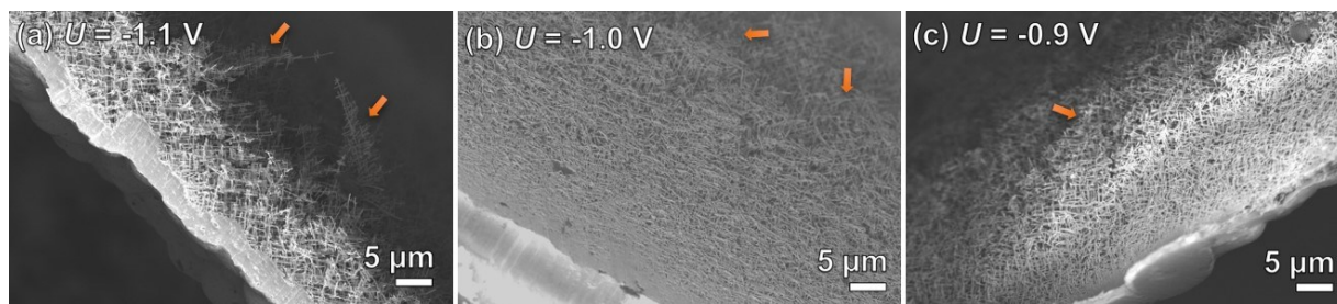
Figure 3.2 SEM images of cross-sections of Au NWNW deposited at (a) U = -1.1 V, (b) U = -1.0 V (c) U = -0.9 V vs. Ag/AgCl. The orange arrows indicate some branches of nanowires grow higher than average, and the inhomogeneity decrease, from a to c, as the deposition potential is less negative.
