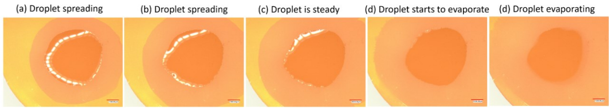
Figure 5.9 Photos of a 5 \mu\text{L} droplet on top of a hydrophilic nanowire network sample by Keyence optical microscope, a wetted ring around the droplet can be observed, scale bar is 1 mm. Nanowire diameter 120 nm, density 1.3 \times 10^9 \text{ cm}^{-2} , with porosity of 74%.
