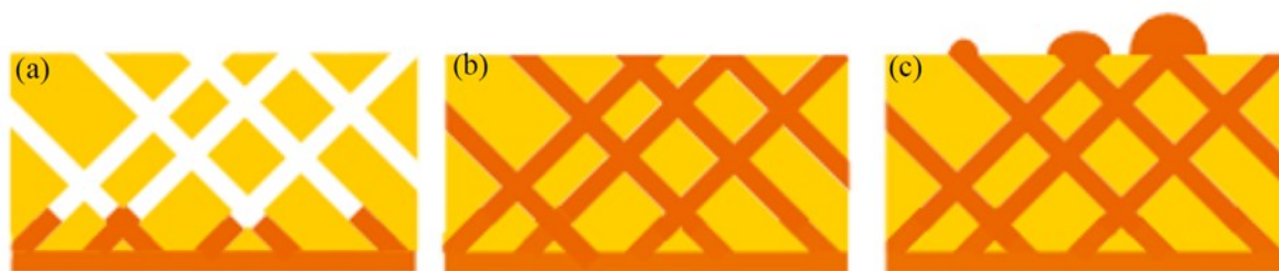
Figure 2.7 Schematic drawing of the deposition process of nanowire networks. 80
