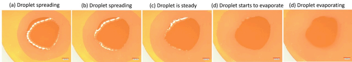
Figure 5.9 Photos of a 5 \mu\text{L} droplet on top of a hydrophilic nanowire network sample by Keyence optical microscope, a wetted ring around the droplet can be observed, scale bar is 1 mm. Nanowire diameter 120 nm, density 1.3 \times 10^9 \text{ cm}^{-2} , with porosity of 74%.
