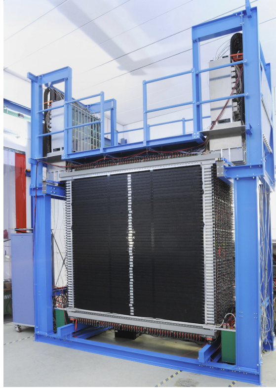
Figure 2.7.: NeuLAND at R^3B with 13 double planes. Figure taken from [75].
