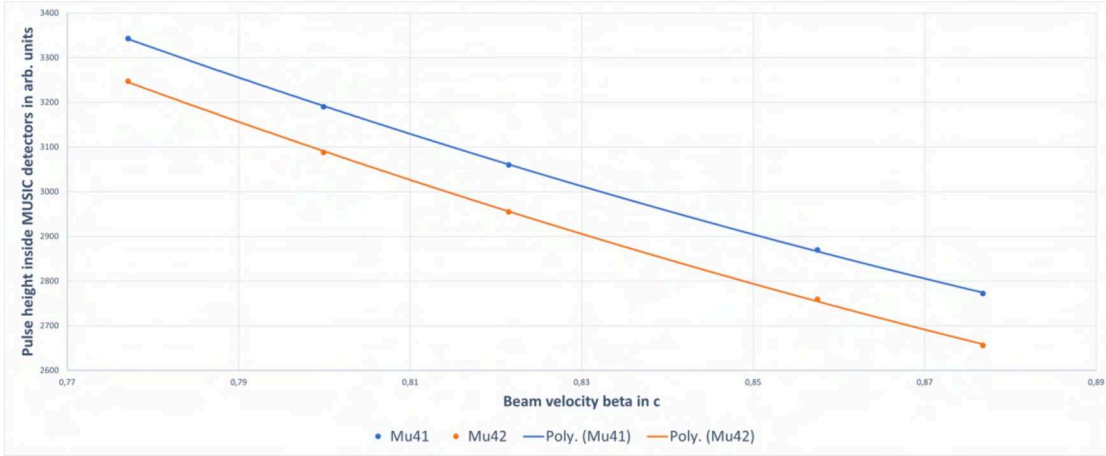
Figure 5.1: Velocity Calibration of MUSIC41 in orange and MUSIC42 in blue. The pulse height of the MUSIC detectors were measured at five different velocities of the primary beam. The results of this measurement are shown in the Tabela 5.2. Second order polynomials were fitted to determine the calibration factors (Table 5.3).
