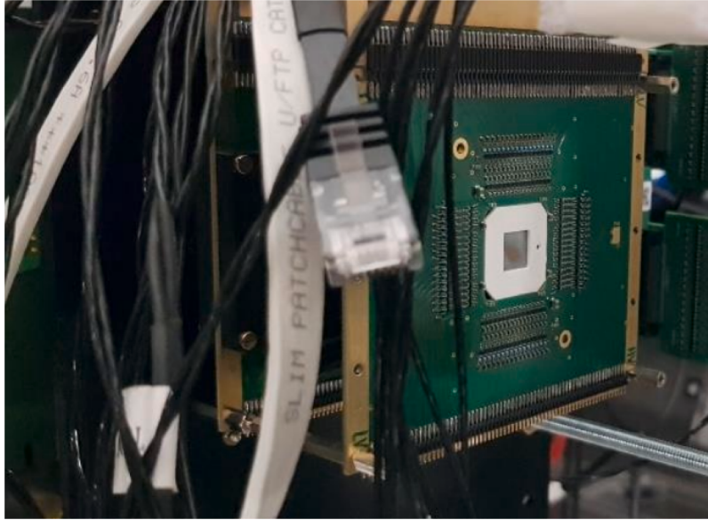
Fig. 4. LGAD sensor mounted on the AC-coupled front end board.
