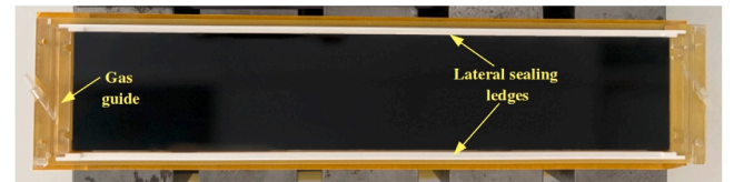
Fig. 3. The two ledges positioned parallel to the long sides of the glass plates and the two gas guiders installed at the two ends for gas inlet and outlet.
