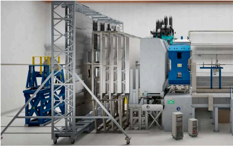
Figure 1. Rendering of the CBM experiment, with the large blue dipole magnet housing the Silicon Tracking System (STS) at its core, surrounded by additional detector systems. (© GSI/FAIR, Zeitrausch)
