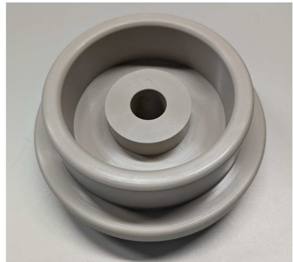
Figure 4: Physical condition of the PEEK-inlet after high-power conditioning in top view.
