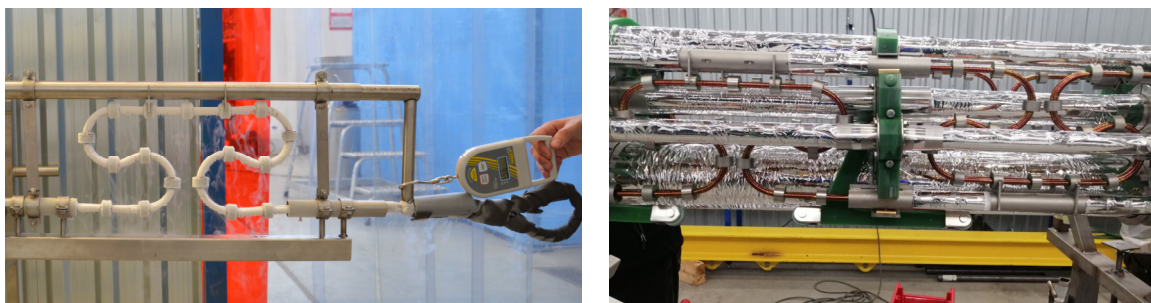
Figure 3. Compensation lyre for the compensation of the thermal shrinkage; left test set-up, right realisation for the 4 pairs of bus bar integrated in the BPL module.
