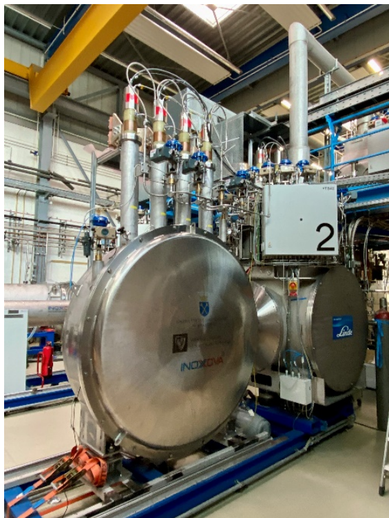
Figure 3: The FOS current lead box at cold testing at the GSI series test facility (STF).
