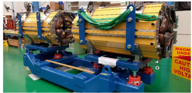
Figure 1: Radiation hard quadrupole magnets for the SIS100 extraction straight at FAT at Buckley, New Zealand.
