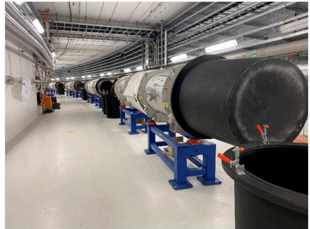
Figure 4: S.c. dipole pairs after installation one of the arcs.
