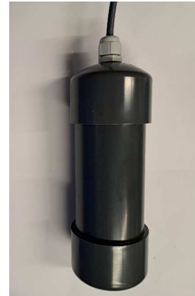
Fig. 2. Example of casing containing the \gamma -detector and ancillary sensor. The length is approximately 10 cm and stands water pressure up to 3 m.
