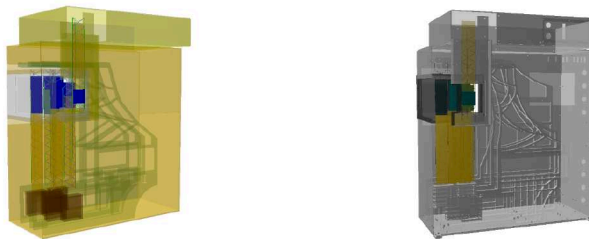
Figure 5. mSTS simulation geometry based on primitive solids (Left) and tessellated solid (right) used in the simulation.
