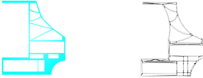
Figure 3. Support structure for ladder called C-frame prepared using primitive solids (Left) and directly from a CAD into ROOT (Right).
