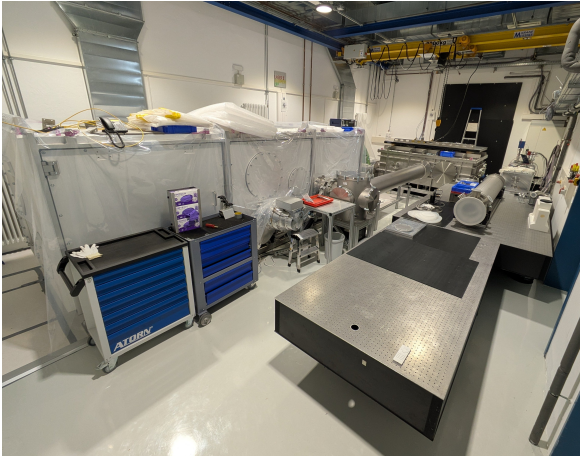
Figure 1: View into the POLARIS compressor laboratory. The vacuum system is located in the left rear area and the optical tables are on the right.
