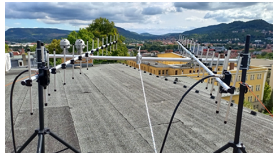
Figure 2: Two Yagi antennas on the roof of the Institute for Solid State Physics in Jena, oriented towards Dresden.
