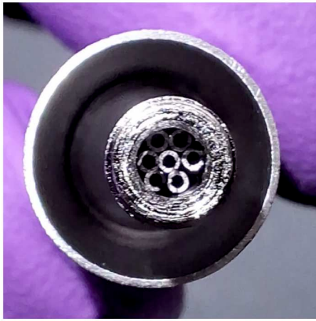
Fig. 7. Photograph of the multi-capillary atom source, corresponding to model B in Fig. 5. The individual capillaries are placed inside a standard RISIKO source. The larger cylinder visible around serves as a heat screen during operation and is not an active part of the atom source.
